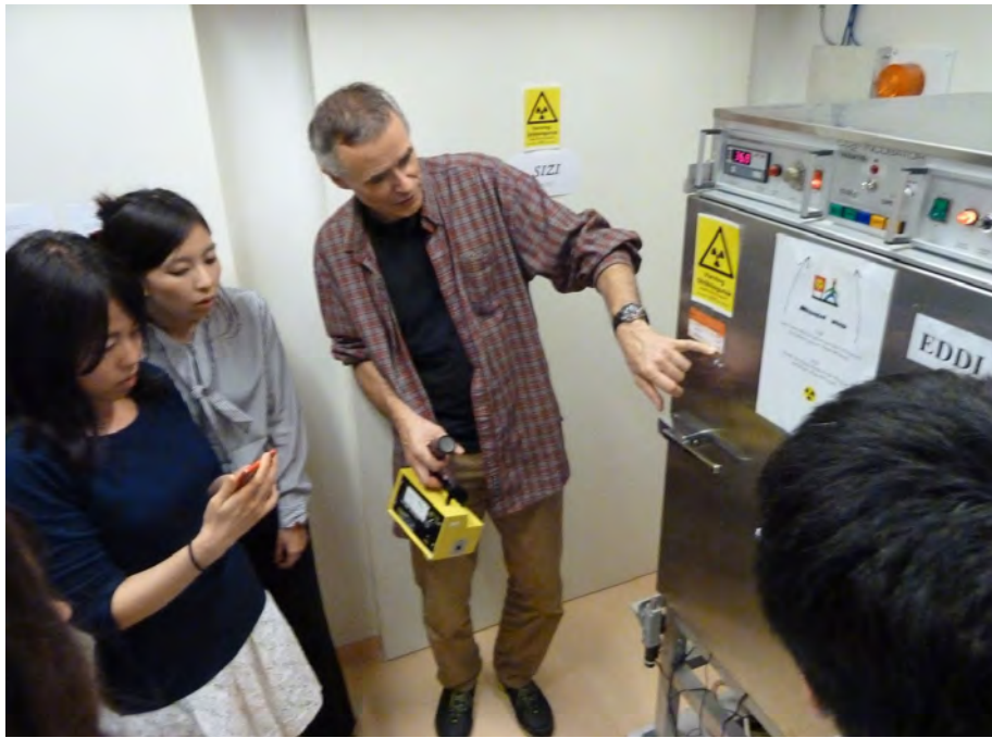
Prof. A. Wojcik was introducing the low dose rate (mGy/h) gamma incubator (Cs-137 source).
