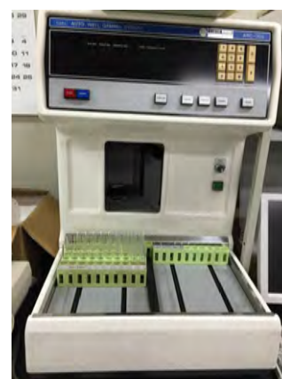
Measuring ^{137}\text{Cs} by an Nal scintillation counter
