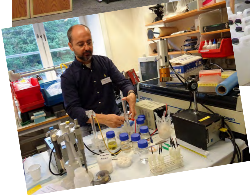
Simulated setting up of an electrodeposition cell for uranium alpha source preparation
